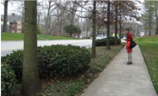
Planting strips accommodate a variety of vegetation that should help separate pedestrians from traffic, define the character of the overall street, enhance adjacent buildings and open space, and allow natural stormwater infiltration.
