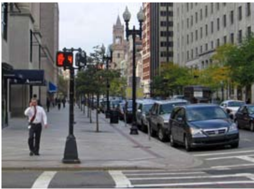
Countdown crossing signals alert pedestrians to remaining safe crossing time more effectively than simple flashing signals.
