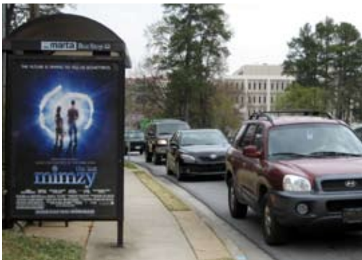
Provide sufficient sidewalk width so that bus shelters do not crowd walking area.
