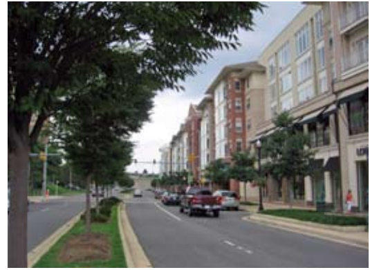
This street in Arlington, Virginia, suggests how Clifton could look along the Emory Point project. Well-articulated buildings define the street edge and add residential and retail activity; median and side planting strips create room for canopy trees and shrubs and reduce paved surface; and on-street parking serves retail and helps buffer pedestrians from traffic.
