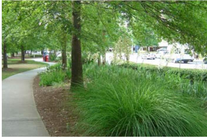
Planting strips accommodate a variety of vegetation that should help separate pedestrians from traffic, define the character of the overall street, enhance adjacent buildings and open space, and allow natural stormwater infiltration.
