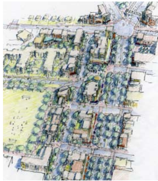
Creating a street grid with multiple circulation choices is one of the most effective ways of reducing traffic congestion.
